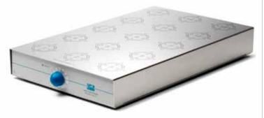
The **MULTISTIRRER Digital** provides synchronized stirring on 6 or 15 samples. A **digital display** ensures a precise setting of stirring speed, constantly. One of its most appreciated features, in microbiology and biochemistry, is that it **remains cold**. Its versatility is extended by the possibility to be combined with a recirculating water bath to thermostat the samples.
